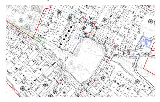
Image above from Phase 3 Drainage Layout displays onsite watercourse routing, notably between Arable Close and Ferguson Road. It is unclear from publicly available site plans where the watercourse has been culverted, and where the watercourse is unculverted.
